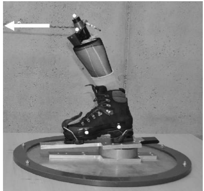
Fig. 1. Measurement of boot shaft stiffness. A load, indicated with the white arrow, was applied on top of the prosthesis fit into the boot. The load, elongation of the top of the prosthesis as well as the moment arm of the load with respect to the ankle joint centre was measured.
